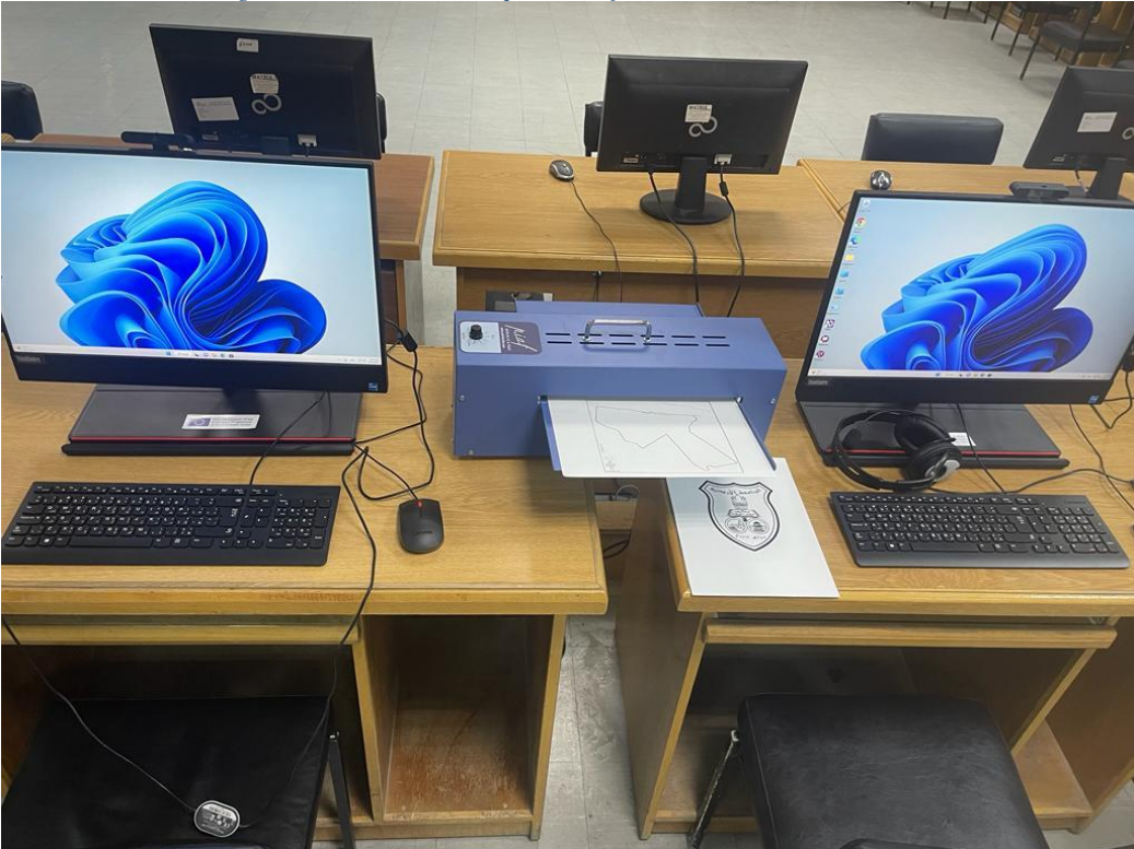
Figure 7. Installation and operation of AT ttols in the AU (PIAF tactile printer)
