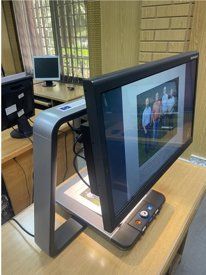
Figure 5. Installation and operation of AT tools in the AU (OCR and magnifier)
